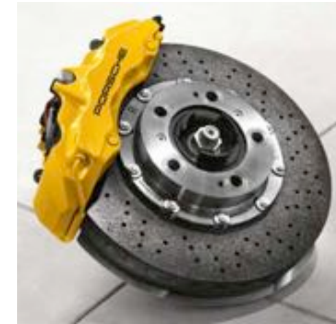
Porsche Ceramic Composite Brake (PCCB)
