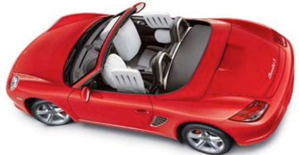
Porsche Side Impact Protection System (POSIP)
